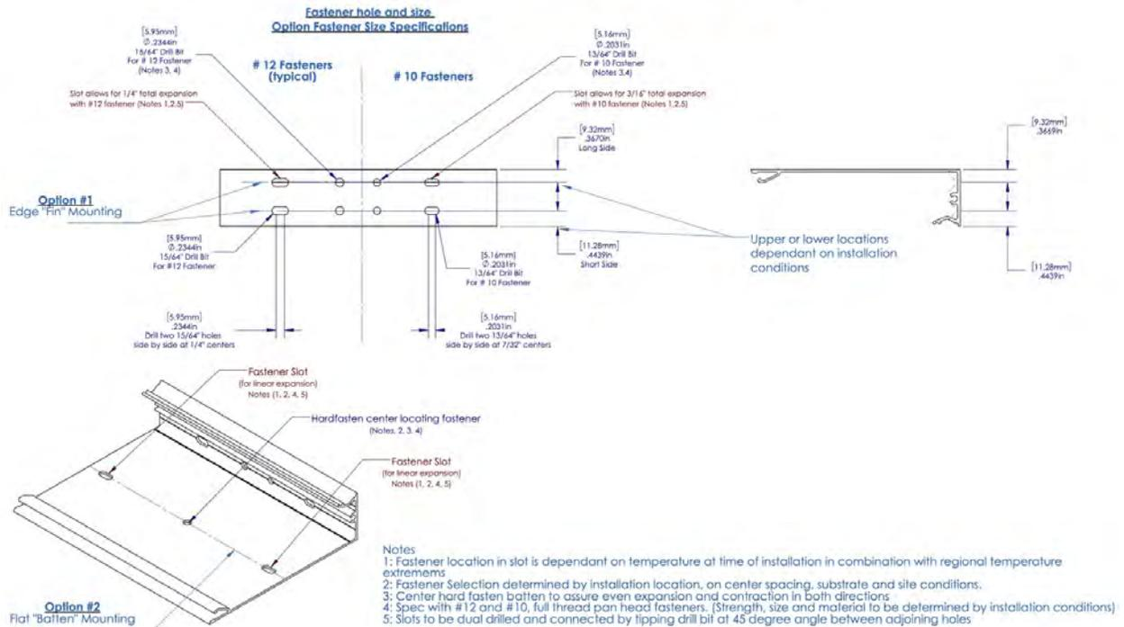
At the time of installation, consider the current temperature as it relates to the expected annual high and low range, to place the fasteners at the slotted holes at either the:
