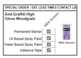
Note: Cleaning the surface with a cleanser that is not diluted as per instructions, may result in damage to the coating.
