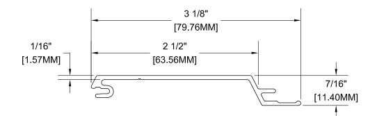
2-1/2" V-GROOVE ALUMINUM ALLOY: 6063-T5 WEIGHT: 0.309 LBS/ LF SCALE: 1:1
