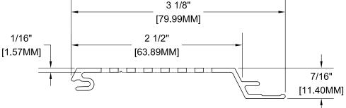
**6" V-GROOVE PERFORATED** ALUMINUM ALLOY: 6063-T5 WEIGHT: 0.447 LBS/ LF the requirements of your particular project. Mayne Coatings Corp. and Longboard products accepts no liability in respect to the use of these drawings. For complete installation instructions refer to the appropriate documentation here NFA: 21% vw.longboardproducts.com/resources/technical-documentation/installation-guides SCALE: 1:1
