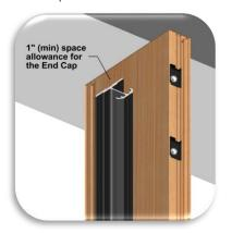
Make sure the Stiffener is located at the end of the back "L" and the tape is in the center of the stiffener.
