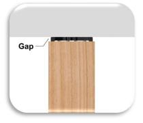
Cut off Taped/Drilled L&L ends (1/2" each end).
