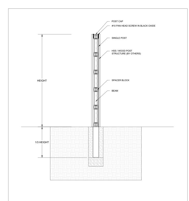
These drawings are published as an information guide only. These CAD drawings are intended as templates to assist the designer, they do not contain the full detail required for construction and must be read in conjunction with the installation instructions on <a href="www.longboardproducts.com">www.longboardproducts.com</a>. You should obtain architectural, engineering or other technical advice to assess the suitability of these drawings to the requirements of your particular project.
