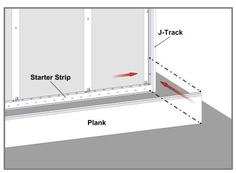
Ensure there is sufficient room for expansion and contraction of each Plank, also confirming component caps will cover.
