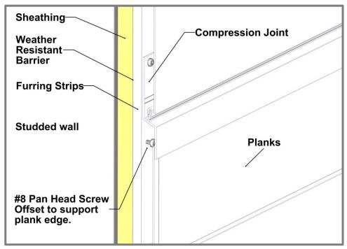
Type: Compression Joint, Termination set/Starter J-Track, J-Track back-to-back.
