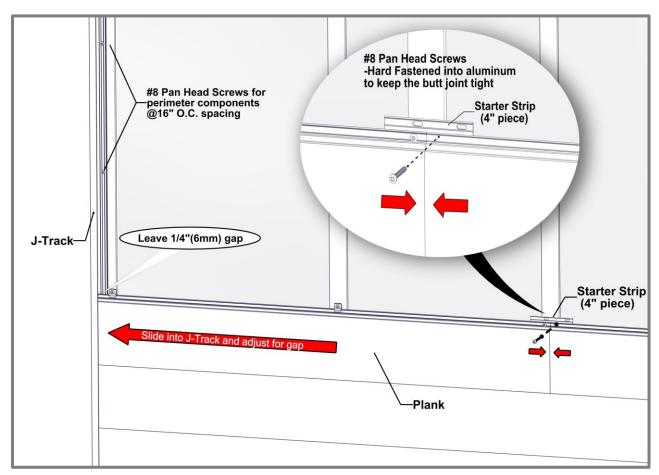
**Detail A -Horizontal Cladding**
