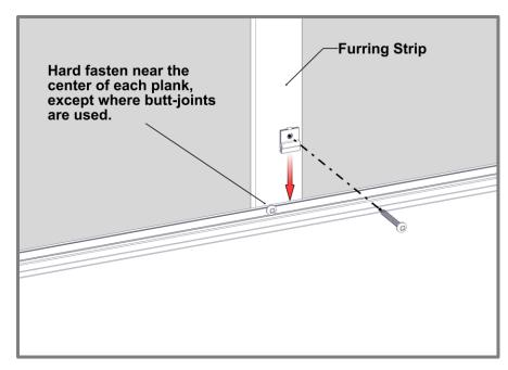
Install planks as needed. Where anchoring the planks securely can only be achieved over component flanges; split the Quick Screen Clip and use one piece on the front.
