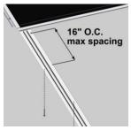
Flat Reveal (Only if required for long runs) Install the Flat Reveal Set base at the desired plank lengths.
