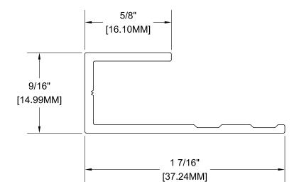
PRECISION J-TRACK (5/8") ALUMINUM ALLOY: 6063-5T WEIGHT: 0.175 LBS/ LF SCALE: 2:1
