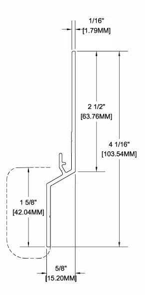
TRADITIONAL COMPRESSION JOINT (1-3/8") ALUMINUM ALLOY: 6063-T5 WEIGHT: 0.418 LBS/ LF **SCALE: 1:1**
