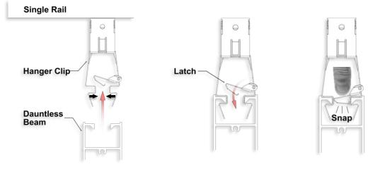
Dauntless Interior Ceiling System Installation Guide
