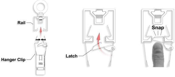
Dauntless Interior Ceiling System Installation Guide
