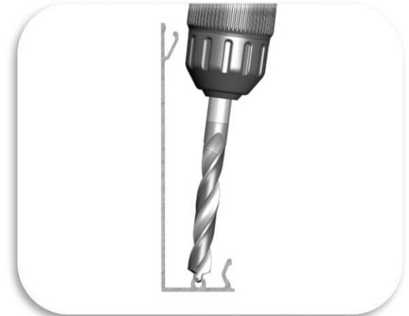
Drilling (Fin orientation)
