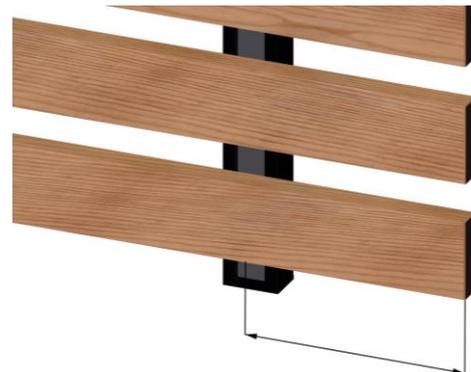
Cantilevers are not to exceed half the allowable span to a maximum of 2'.
