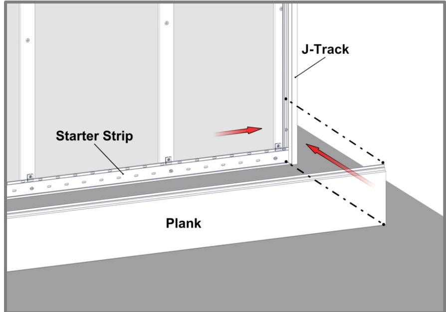
When installing Planks, ensure there is sufficient room for expansion and contraction of each Plank, also confirming component caps will cover.
