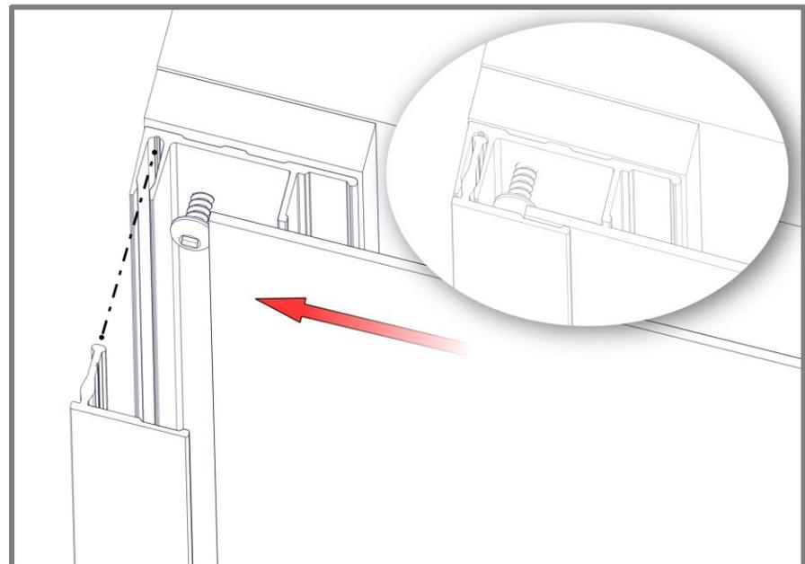
**Finishing Steps** - Once planks are installed, finish off the perimeter trims with caps from two-piece sets.
