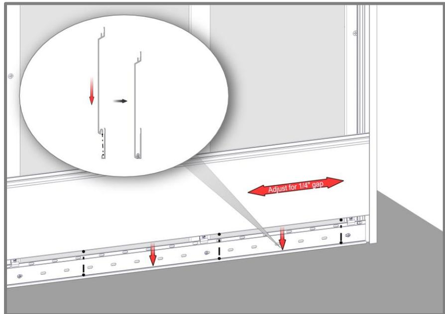
Install Quick Screen Clips every 32" (813mm) O.C. max spacing. Hard fasten only one point at the center of each plank, except where butt-joints are used. Shim Quick Screen Clips where needed to correct any substrate inconsistencies.
