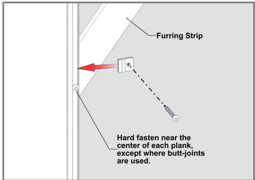
Install planks as needed. Where anchoring the planks securely can only be achieved over component flanges; split the Quick Screen Clip and use one piece on the front. This will maintain each plank's ability to expand and contract.
