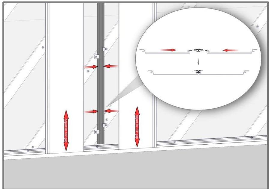
Install Quick Screen Clips every 32" (813mm) O.C. max spacing. Hard fasten only one point at the center of each plank, except where butt-joint are used. Shim Quick Screen Clips where needed to correct any substrate inconsistencies.
