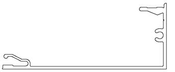
FIGURE 3-LINK & LOCK BATTENS (4-INCH PIECE TUBE AS SHOWN, ALSO AVAILABLE IN 2, 6 AND 8-INCH TUBES)
