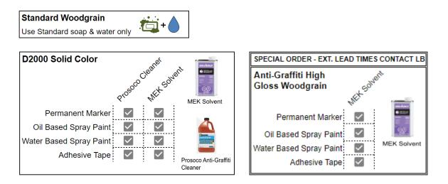
Note: Cleaning the surface with a cleanser that is not diluted as per instructions, may result in damage to the coating.
