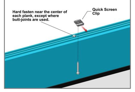
Where anchoring the planks securely can only be achieved over component flanges; split the Quick Screen Clip and use one piece on the front. This will maintain each Planks ability to expand and contract.
